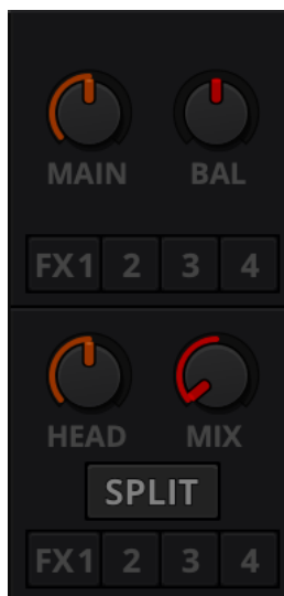
Figure20: The headphone and main mix knobs
