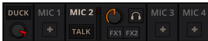
Figure1: The microphone ducking controls
